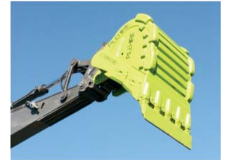
Bucket with cutting edge added
