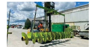
Forklift mounted spreader beams for lifting wide loads
