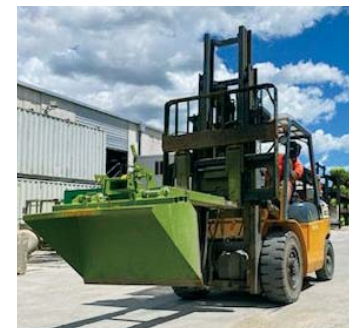
Tipper bucket for forklift, for scrapping up around the yard and dugging
