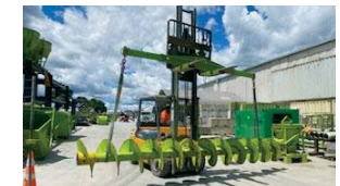
Forklift mounted spreader beams for lifting wide loads
