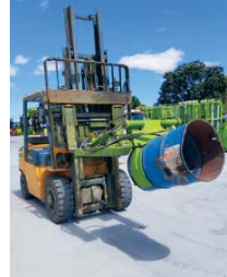
Drum tipper used for tipping drums of oil or emptying bins etc
