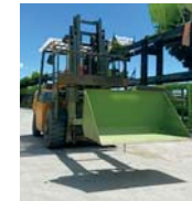
Tipper bucket for forklift, for scrapping up around the yard and dugging
