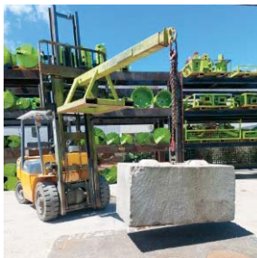
Lift extension for hard to get to and ease of lifting.
