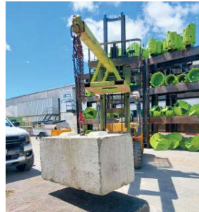
Lift extension for hard to get to and ease of lifting.
