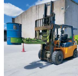
Drum tipper used for tipping drums of oil or emptying bins etc
